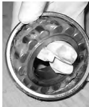
Fig. 10. Grease can easily be packed by hand.
